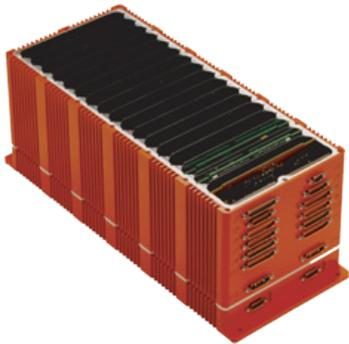
**STANDARD HOUSING WITH COVER REMOVED REVEALS INDIVIDUAL CARD SHIELDING**
